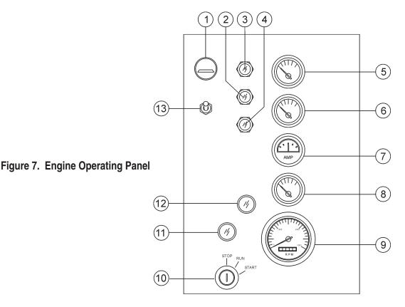
The definitions below describe the controls and functions of the "*Engine Operating Panel*" (Figure 7).
